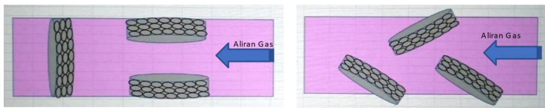
Gambar 7. Ilustrasi Adsorben MEF-20; (a) Vertikal-Horizontal (V-H), (b) Zig Zag
